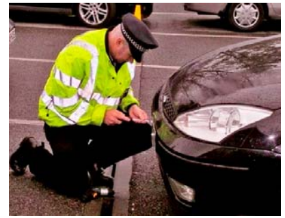
Picture shows the anti-tamper proof screws being fitted.
